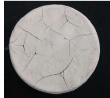
Fig. 5 Mud cake after 3 hours' heating
