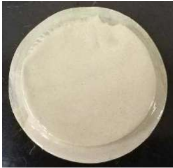
Fig. 4 Mud cake after 0.5 hours' heating
