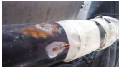
Fig. 12 Stress test of linkage rod
