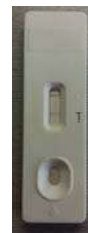
Fig. 2 the detection strips. The bottom area is a sample pad where the reagent of cadmium to be detected drips; the top area is the T-line areas marked by the letter "T".
