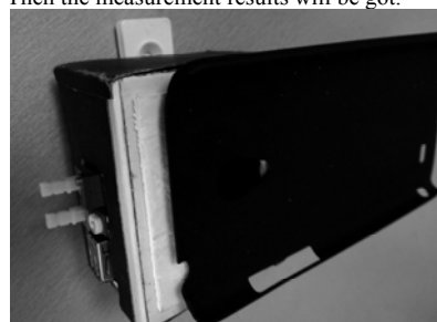
Fig. 3 the environmental device. A groove in the bottom is used for the insertion of the detection strips. A phone cover is employed to fix the phone, making the T line aligned with the camera. LED switch and USB interface are designed in the back.
