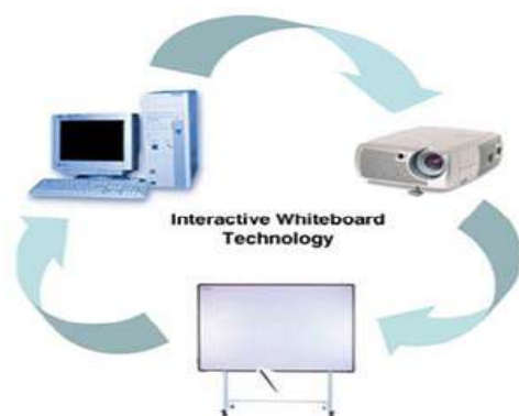
Fig1. The computer images are displayed on the board by the digital projector. The images then can be seen and all applications on the computer can be controlled via touching the board, either with your finger, or with an electronic pen/stylus.
